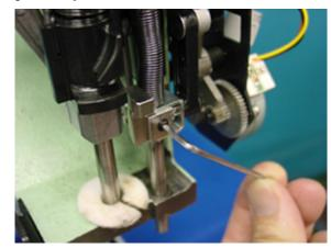
1. Change needle bar to no. 0 and disconnect cable from pulse motor.
