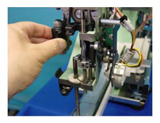
2. Loosen the screw which fixes guide shaft then move the guide shaft lower.
