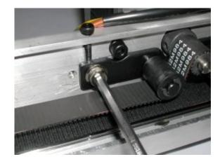
10. Tighten fixing screw for tension pulley bracket. (rear side)
