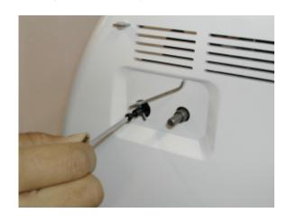
5. Confirm that the shaft does not touch the cover by turning motor.
