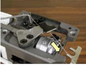
4. Tighten lock nut. (Don't move adjusting screw.)
