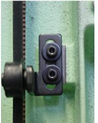
Please move tension shaft ass'y upward and downward to adjust.
