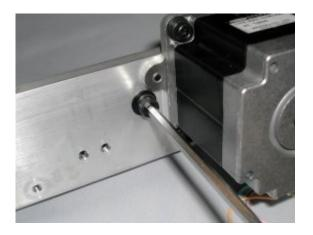
9. Remove belt from motor pulley.
