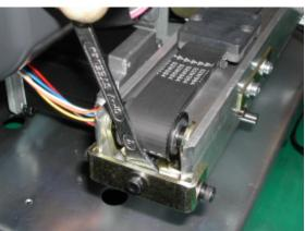
5. Adjust belt tension, to use belt tension gauge.
