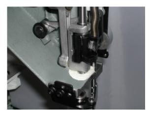
3. When dial disc reads [0 degree], fix detecting disk.
