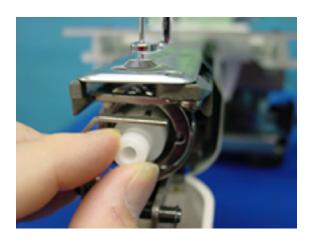
Adjust the needle bar height up and down till the needle tip touches to the gauge slightly.
