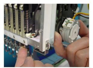
3. Pull pressure foot bracket ass'y downward, then fix it.
