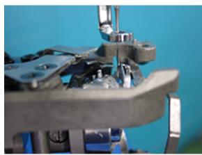
7. For making sure, check position of retainer on bobbin case holder.
