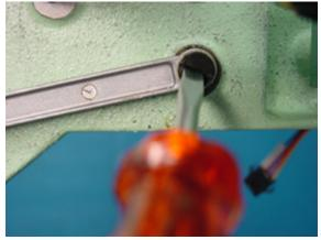
6. Exchange pressure foot drive lever ass'y.
