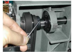
4. Loosen screw on fasten collar for take-up lever cam.
