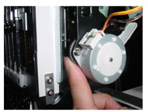
3. Disconnect cable from Sensor board ass'y and Remove bracket ass'y.
