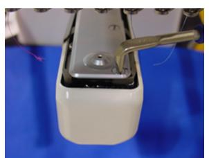
2. Open moving knife, check if knife drive shaft has no backlash in up and down direction.
