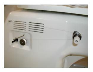
8. Adjust the inclination of Winder bracket ass'y in accordance with thread winding condition.
