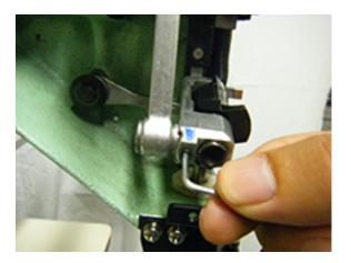
5. Remove needle bar driver ass'y.
