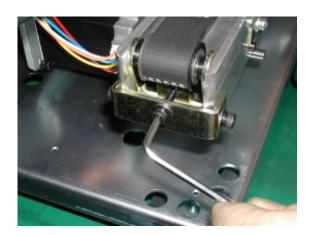
4. Loosen tension screw so as to move tension.
