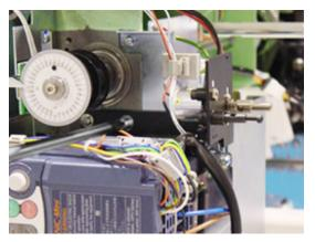
2. Fix 2 screws tentatively timing detecting board.
