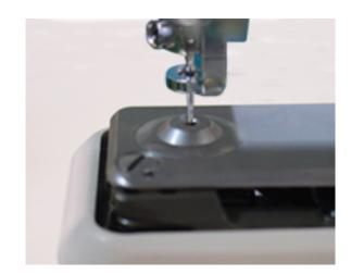
After adjustment, please be sure to check and adjust clearance between needle and shuttle hook.
