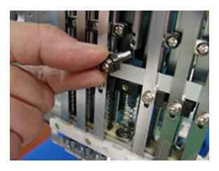
While pressing needle bar spring, insert good needle bar with needle bar boss, needle bar boss B, Pressure foot block B, Cushion, Plain washer (M6), Needle bar spring H and Pressure foot spring.
