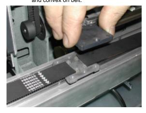
Do not put belt tooth on the innermost groove of the connecting plate.
