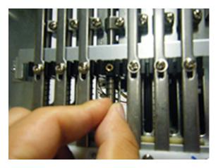
7. Fix needle , needle holder and pressure foot.
