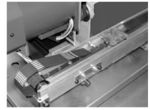
8. Set belt to belt groove of guide frame base.
