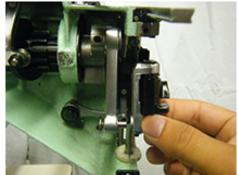
10. Remove circuit board assembly for timing detecting
