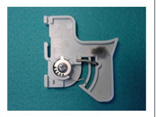
2. The Thread adjusting plate has a latch to be able to adjust tension in three steps.
