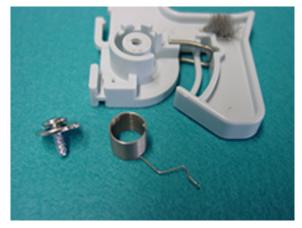
5. Exchange thread adjusting spring.
