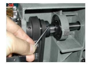
5. Loosen screw on fasten collar for take-up lever cam.
