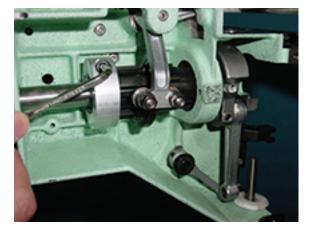
4. Turn take up lever cam slowly and insert positioning pin into pin groove.
