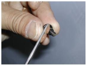
9. Assemble pressure foot drive lever ass'y.
