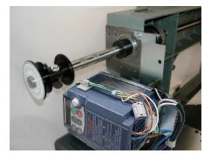
7. Remove upper pulley and timing belt.
