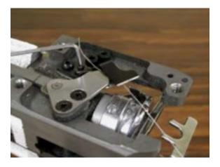
Through height of bobbin thread holder, you can adjust holding power for bobbin thread.
