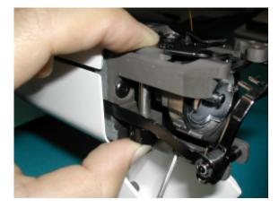
Referring to [3-6-8 Adjustment of moving knife and fixed knife],check how well thread is cut and adjust, then finish this process.
