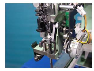
Adjust the height of pressure foot guide bar to finish.
