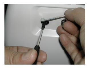
9. Remove cover (left). (Remove screw in arrow mark)
