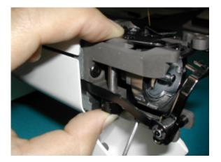
3. Adjust slant of fixed knife with [upper adjustment screw] and [lower adjustment screw] that fix fixed knife.
