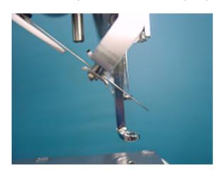
If you can not set the correct position with procedure no.4, then Thread catcher device should be adjusted.
