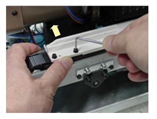
Hold the right side of arm to arrow pointed direction at below picture and tighten screw.
