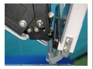
2. Insert needle bar boss B into block ass'y, then insert forked part of take-up lever into take-up lever guide bar.
