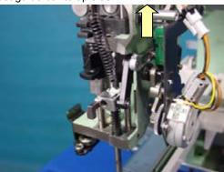
5. Remove pressure foot drive lever ass'y
