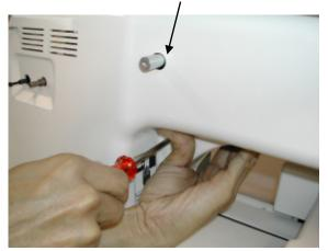
3. Assemble thread tension ass'y.
