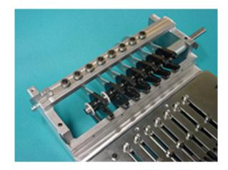
Leave space of [0.03mm] between take-up lever and moving head, then set the E-ring.
