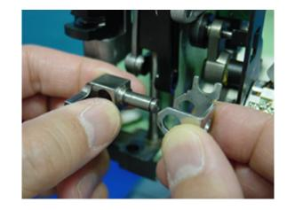
5. Assemble the pressure foot gude bar and Pressure foot spring.
