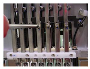
After adjustment, when pressing pressure foot to bottom with hand, confirm whether pressure foot turns back by spring.  Referring to [3-2-1 Exchange of crank], remove Front coverand Thread tension.
