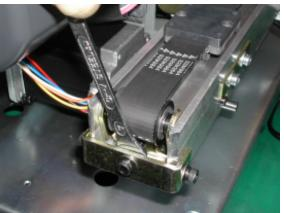
4. Loosen tension screw so as to move tension.
